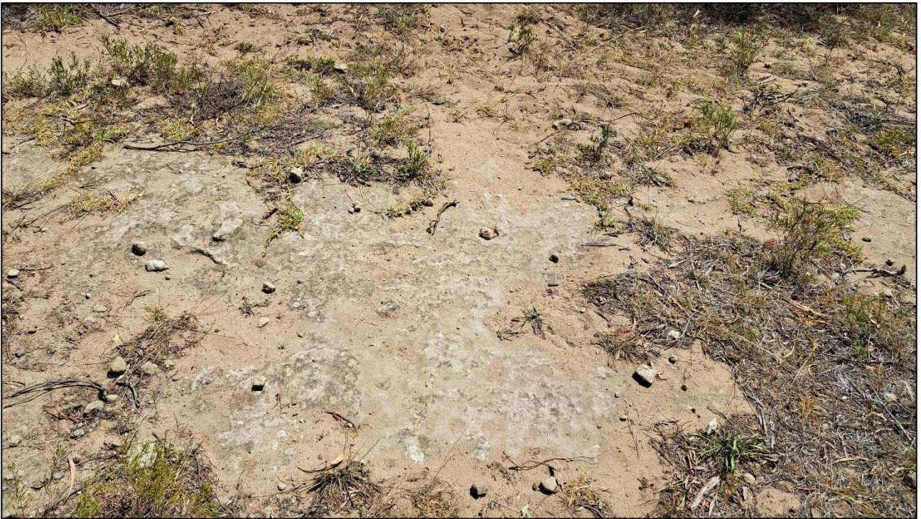
Figure 17: This exposure of a hard cemented outcrop appears to be a remnant of previous construction activities rather than natural geological formations, as suggested by historical images of the area. The distinct lack of typical sedimentary layering and the presence of scattered debris further support that this feature is anthropogenic in origin. Point 30.
